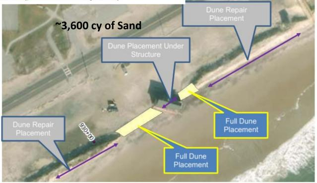
Figure 2: Plan view dune placement schematic.
