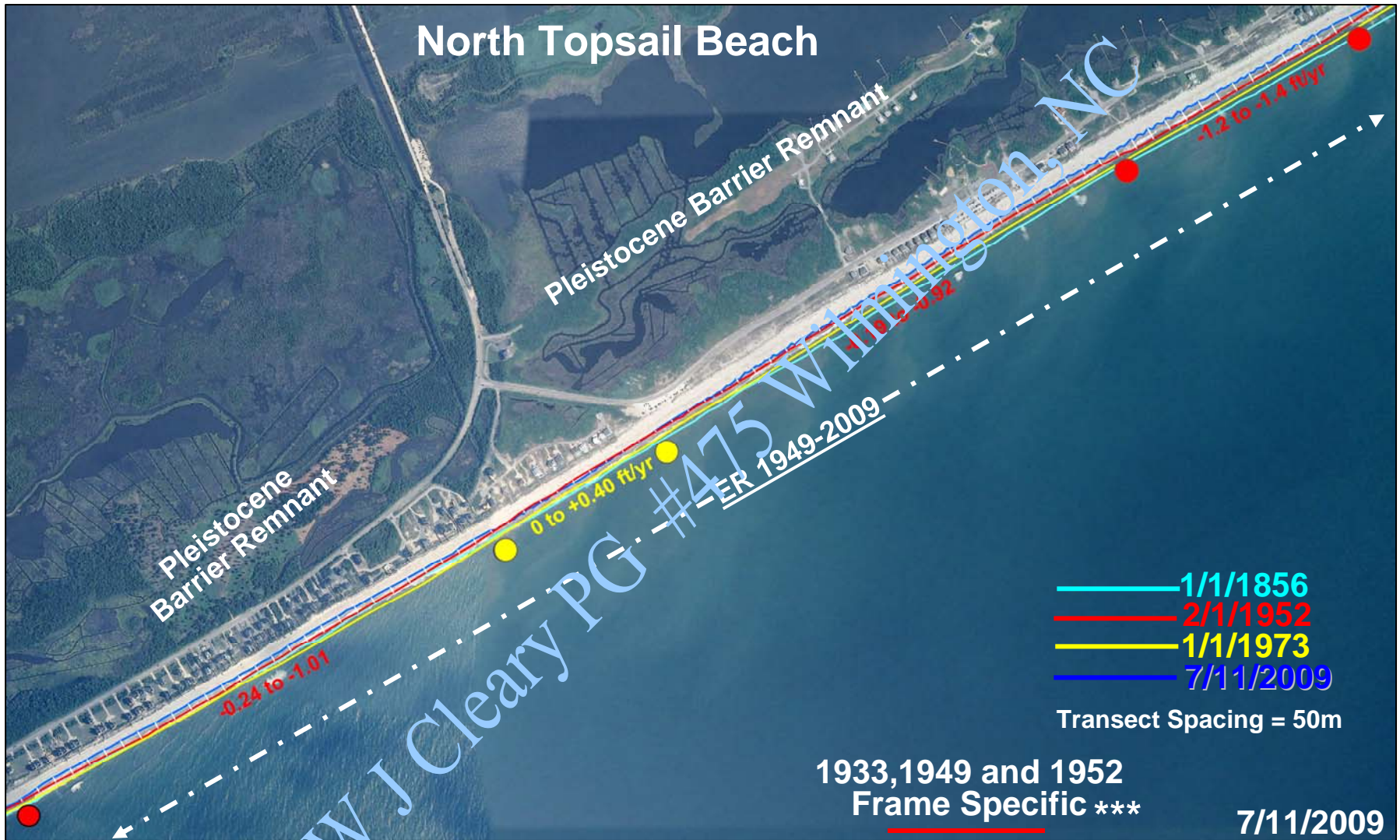
Figure 24. Map depicting 7/11/2009 photograph of the segment located immediately southwest of Figure 23 with NC DCM transects used for measuring erosion rates (2011 updated). Shoreline change rates reflect changes between 1949-2009. Transect spacing = 50m. Data derived from NC DCM's Oceanfront Setback Factor Portal and available GIS files from 2013 (transects 50m shapefile, 2009 shr1 shapefile and Early shr1 shapefile (composite shr1 file for 1933, 1949 and 1952). Additional information was provided by Ken Richardson (NC DCM). http://portal.ncdenr.org/web/cm/oceanfront-construction-setback .
