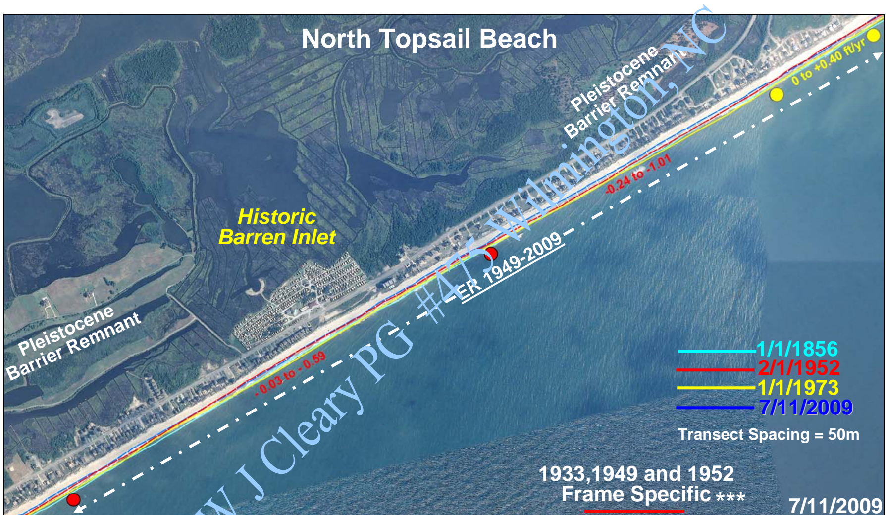
Figure 25. Map depicting 7/11/2009 photograph of the segment located immediately southwest of Figure 24 with NC DCM transects used for measuring erosion rates (2011 updated). Shoreline change rates reflect changes between 1949-2009. Transect spacing = 50m. Data derived from NC DCM's Oceanfront Setback Factor Portal and available GIS files from 2013 (transects 50m shapefile, 2009 shrll shapefile and Early shrll shapefile (composite shrll file for 1933, 1949 and 1952). Additional information was provided by Ken Richardson (NC DCM). http://portal.ncdenr.org/web/cm/oceanfront-construction-setback .
